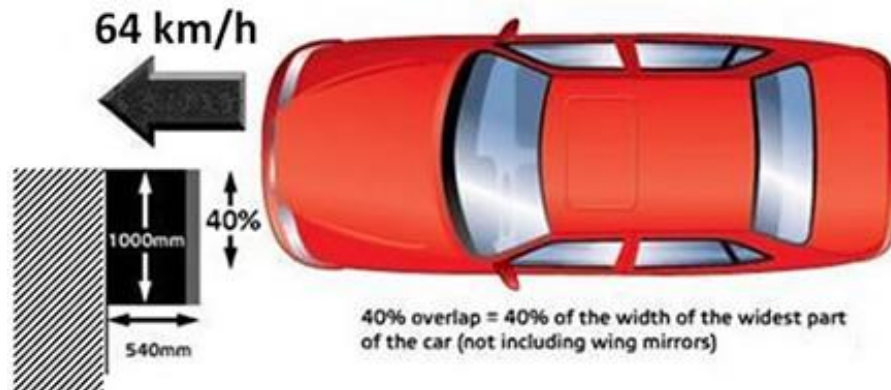
Figura 10 – Esquema representativo do teste de impacto frontal moderate overlap
