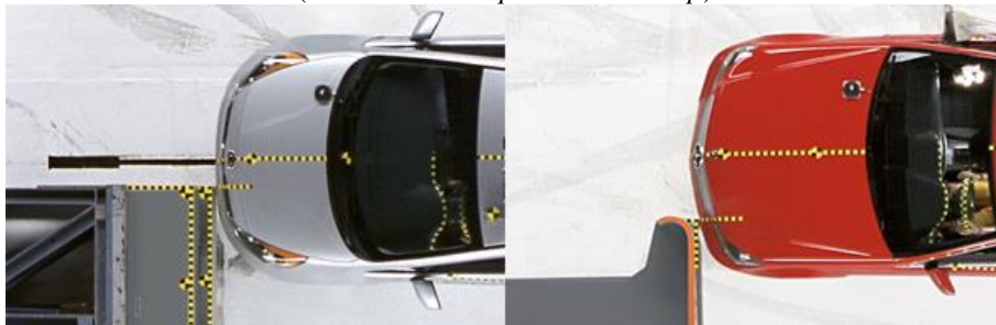
Figura 14 – Vista superior com comparativo entre os padrões de crash tests frontais ( moderate overlap e small overlap )
